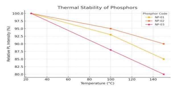
Here is the graph showing the thermal stability of phosphors, illustrating the relative PL intensity (%) at different temperatures.
