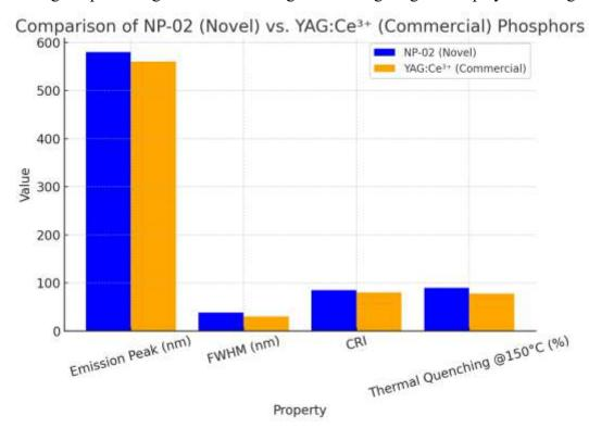
Here is the bar chart comparing NP-02 (Novel) with YAG:Ce<sup>3+</sup> (Commercial) across different photoluminescence properties.
