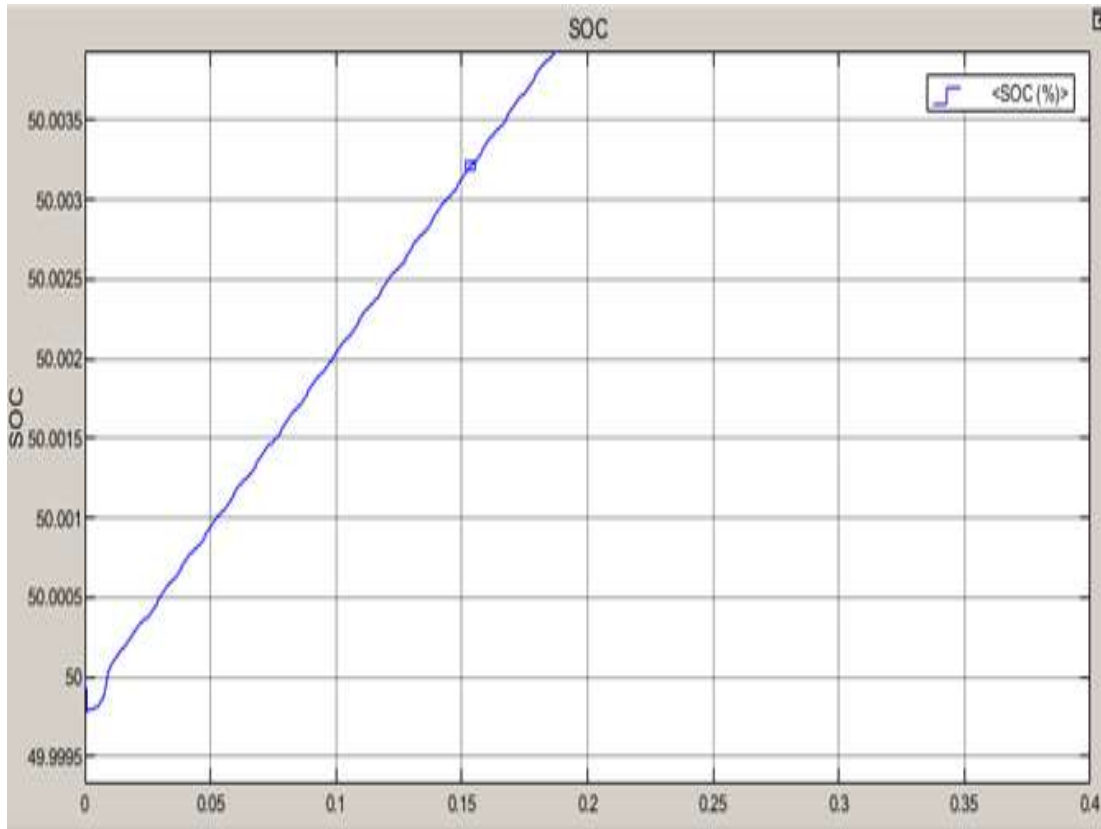
Fig.8 SOC charging at 50%
